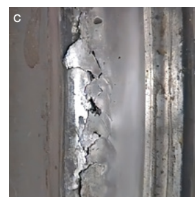
Examples of hydrogen wear on various surfaces. a. Hydrogen wear on an SKF bearing ball, b. and c. A railway wheelset that's been worn down by the absorption of hydrogen during the braking process
