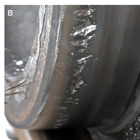
Examples of hydrogen wear on various surfaces. a. Hydrogen wear on an SKF bearing ball, b. and c. A railway wheelset that's been worn down by the absorption of hydrogen during the braking process
